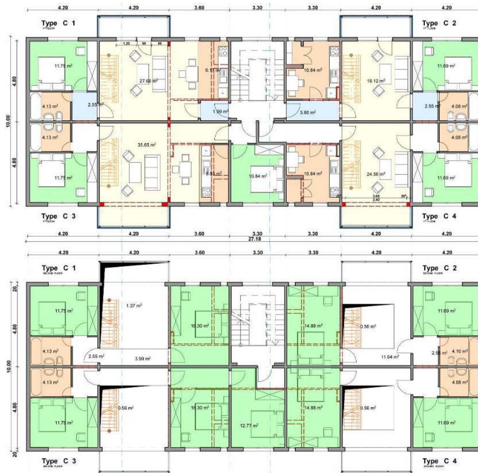
Figure 23: Vertical reconfiguration – creating openings in floors
