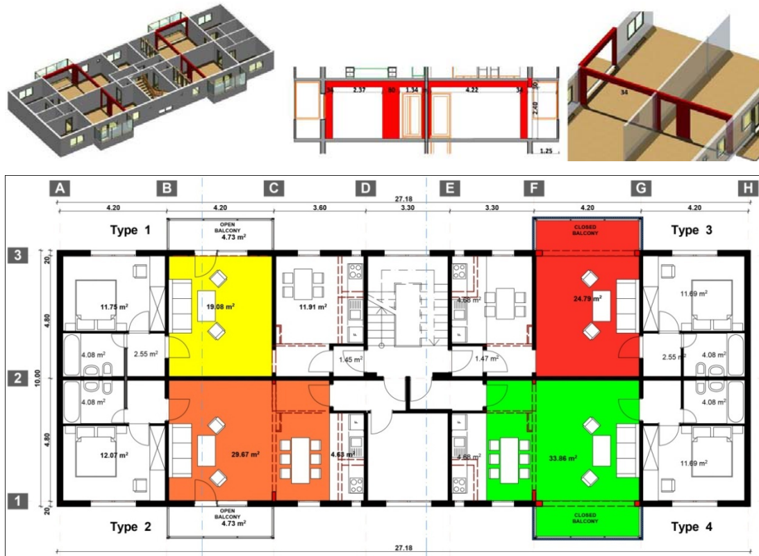
Figure 21: Reconfiguration through replacing walls with steel frames (Botici et al, 2012)
