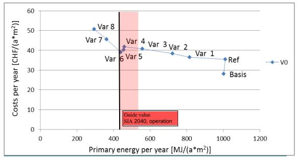
Figure 53: Yearly costs as a function PE efficiency increase due to the strategy steps of the "LCC, PE and GHG optimizer" strategy compared to guide value "operation" and "operation+construction" of SIA 2040.
