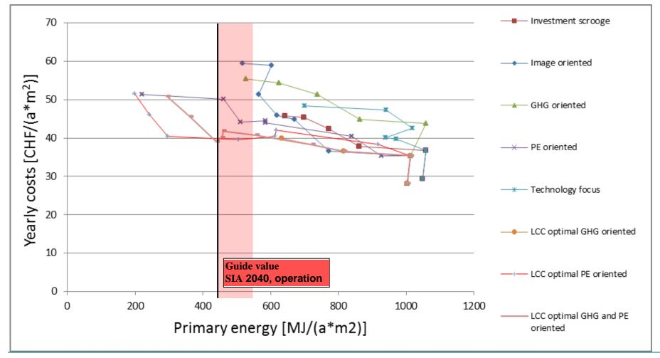
Figure 59: Yearly costs as a function of PE use due to the strategy steps of the each main strategy (applied to the base case building from the construction period 1975-1990) compared to guide value "operation" and "operation+construction" of SIA 2040
