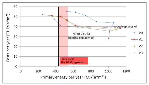
Figure 31: Yearly costs as a function of PE use due to the strategy steps of the each strategy variant compared to guide value "operation" and "operation+construction" of SIA 2040.
