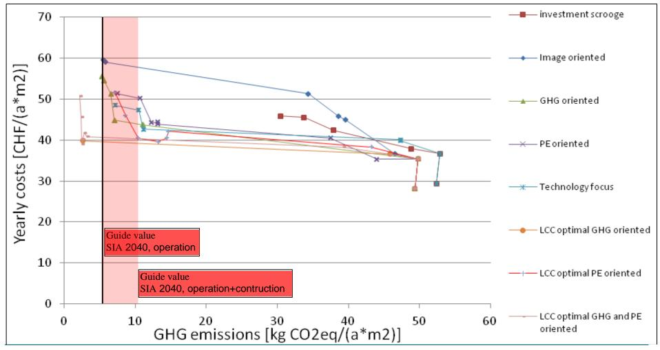
Figure 1: Yearly costs as a function of **GHG emissions** due to the strategy steps of the each main strategy (applied to the base case building from the construction period 1975-1990). The guide value of SIA 2040 is set for operation and the band is until the guide value which includes operation and construction.
