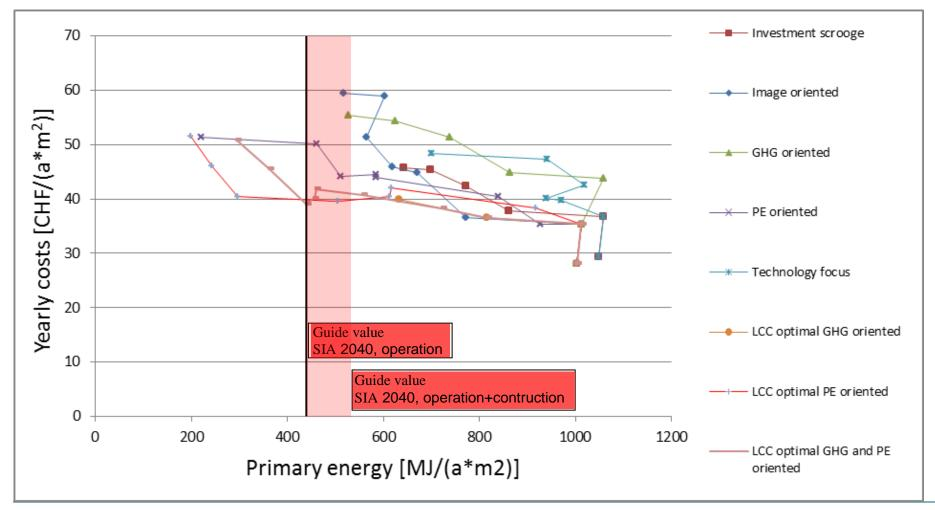
Figure 2: Yearly costs as a function of **primary energy use** due to the strategy steps of the each main strategy (applied to the base case building from the construction period 1975-1990). The guide value is set for operation and the band is until the guide value which includes operation and construction.
