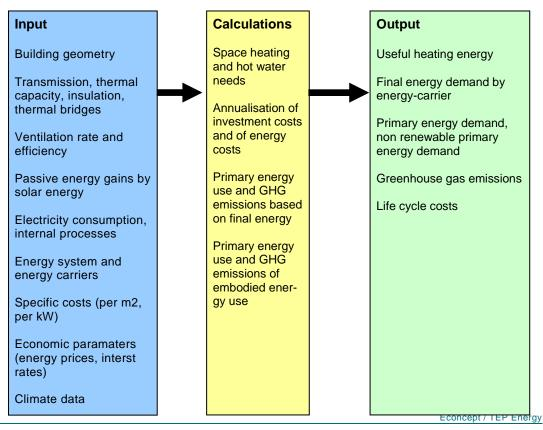
Figure 7: Simplified model representation of used methodology
