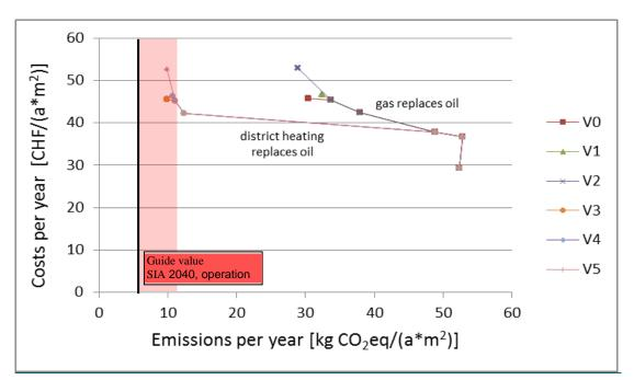
Figure 20: Yearly costs as a function of GHG emissions due to the strategy steps of the each strategy variant compared to guide value "operation" and "operation+construction" of SIA 2040.
