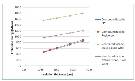
Figure 14: Embodied energy of a compound and ventilated façade insulation with different materials
