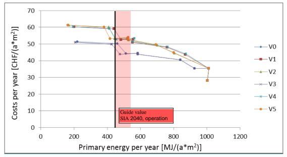
Figure 36: Yearly costs as a function of PE use due to the strategy steps of the each strategy variant compared to guide value "operation" and "operation+construction" of SIA 2040.
