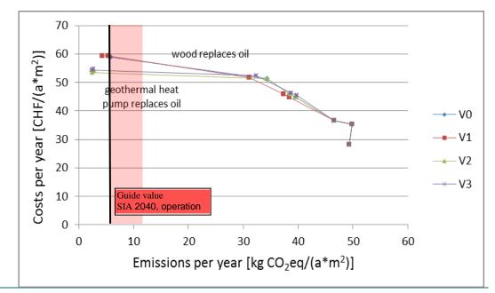
Figure 25: Yearly costs as a function of GHG emissions due to the strategy steps of the each strategy variant compared to guide value "operation" and "operation+construction" of SIA 2040.
