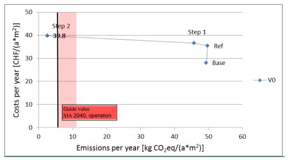
Figure 42: Yearly costs as a function of GHG emissions due to the strategy steps of the "LCC and GHG optimizer" strategy compared to guide value "operation" and "operation+construction" of SIA 2040.
