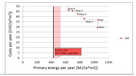
Figure 18: Yearly costs as a function PE efficiency increase due to the strategy steps of the "investment scrooge" strategy compared to guide value "operation" and "operation+construction" of SIA 2040.
