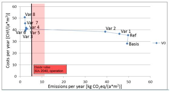
Figure 52: Yearly costs as a function of GHG emissions due to the strategy steps of the "LCC, PE and GHG optimizer" strategy compared to guide value "operation" and "operation+construction" of SIA 2040.
