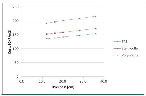
Figure 8: Investment costs of compound façade insulation measures as a function insulation thickness
