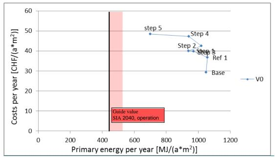
Figure 38: Yearly costs as a function PE efficiency increase due to the strategy steps of the "technology focus" strategy compared to guide value "operation" and "operation+construction" of SIA 2040.
