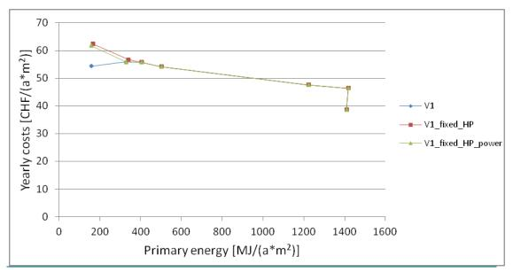
Figure 65: Yearly costs as a function of PE use due to the strategy steps of the strategy (applied to the base case building from the construction period 1947-1975)
