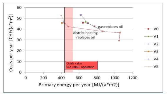
Figure 21: Yearly costs as a function of PE use due to the strategy steps of the each strategy variant compared to guide value "operation" and "operation+construction" of SIA 2040.
