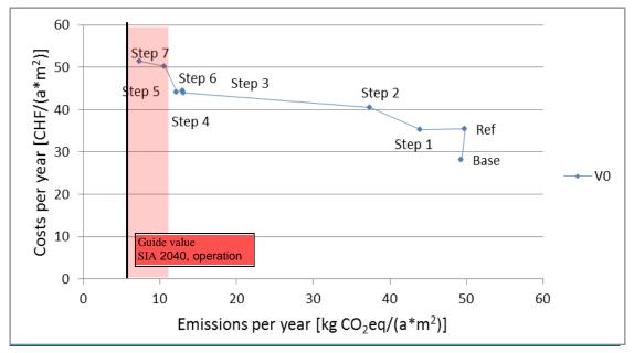
Figure 32: Yearly costs as a function of GHG emissions due to the strategy steps of the "PE oriented" strategy compared to guide value "operation" and "operation+construction" of SIA 2040.
