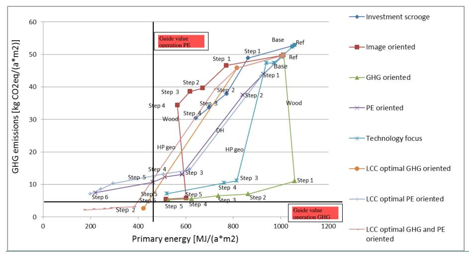
Figure 57: GHG emissions as a function of PE use due to the strategy steps of the each main strategy (applied to the base case building from the construction period 1975-1990) compared to guide value "operation" and "operation+construction" of SIA 2040
