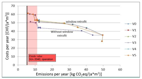
Figure 35: Yearly costs as a function of GHG emissions due to the strategy steps of the each strategy variant compared to guide value "operation" and "operation+construction" of SIA 2040.
