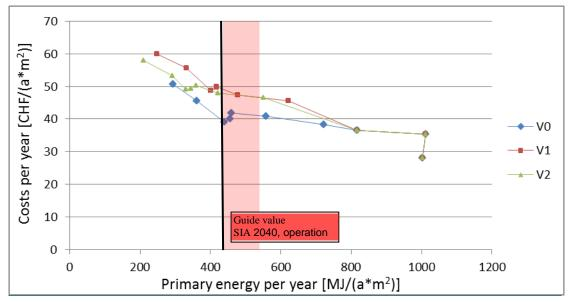
Figure 56: Yearly costs as a function of PE use due to the strategy steps of the each strategy variant compared to guide value "operation" and "operation+construction" of SIA 2040.
