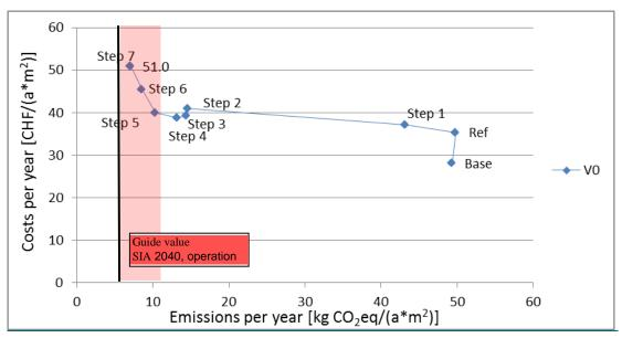
Figure 47: Yearly costs as a function of GHG emissions due to the strategy steps of the "LCC and PE optimizer" strategy compared to guide value "operation" and "operation+construction" of SIA 2040.
