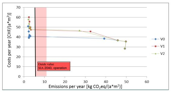
Figure 55: Yearly costs as a function of GHG emissions due to the strategy steps of the each strategy variant compared to guide value "operation" and "operation+construction" of SIA 2040.
