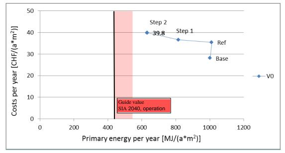
Figure 43: Yearly costs as a function PE efficiency increase due to the strategy steps of the "LCC and GHG optimizer" strategy compared to guide value "operation" and "operation+construction" of SIA 2040.
