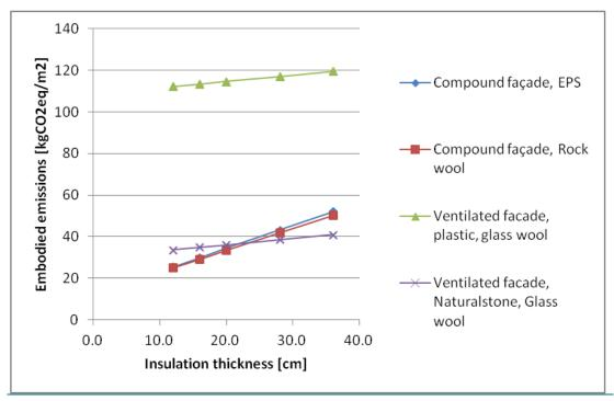
Figure 15: Embodied emissions of a compound and ventilated façade insulation with different materials
