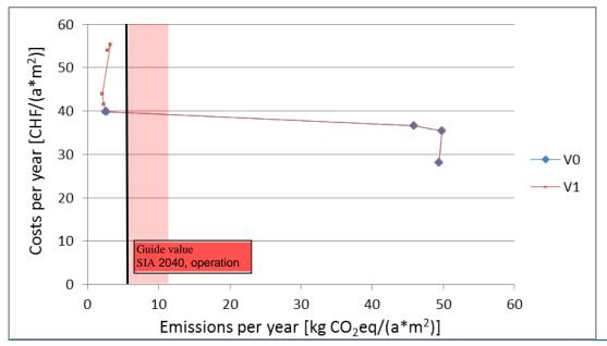
Figure 45: Life cycle costs as a function of GHG emissions due to the strategy steps of the each strategy variant compared to guide value "operation" and "operation+construction" of SIA 2040.
