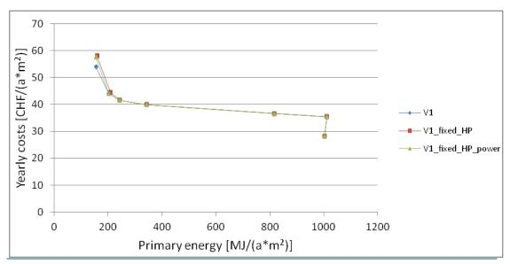
Figure 63: Yearly costs as a function of PE use due to the strategy steps of the strategy (applied to the base case building from the construction period 1975-1990)
