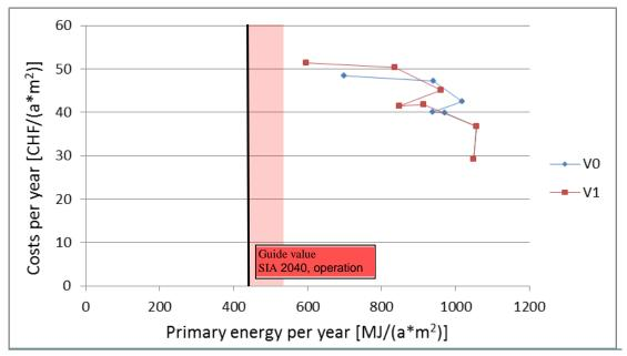
Figure 41: Yearly costs as a function of PE use due to the strategy steps of the each strategy variant compared to guide value "operation" and "operation+construction" of SIA 2040.
