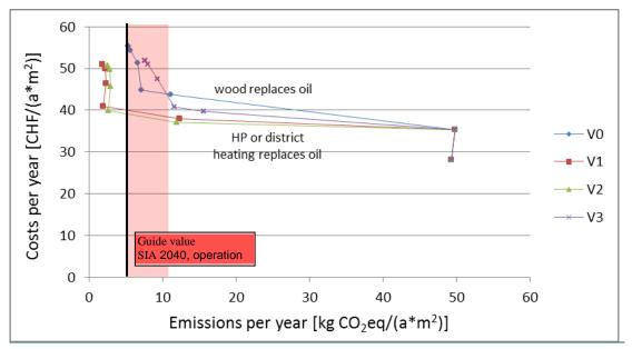
Figure 30: Yearly costs as a function of GHG emissions due to the strategy steps of the each strategy variant compared to guide value "operation" and "operation+construction" of SIA 2040.
