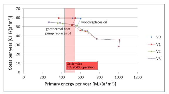
Figure 26: Yearly costs as a function of PE use due to the strategy steps of the each strategy variant compared to guide value "operation" and "operation+construction" of SIA 2040.
