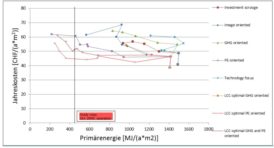
Figure 61: Yearly costs as a function of PE use due to the strategy steps of the each main strategy (applied to the base case building from the construction period 1947-1975)
