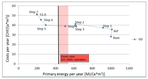
Figure 48: Yearly costs as a function PE efficiency increase due to the strategy steps of the "LCC and PE optimizer" strategy compared to guide value "operation" and "operation+construction" of SIA 2040.
