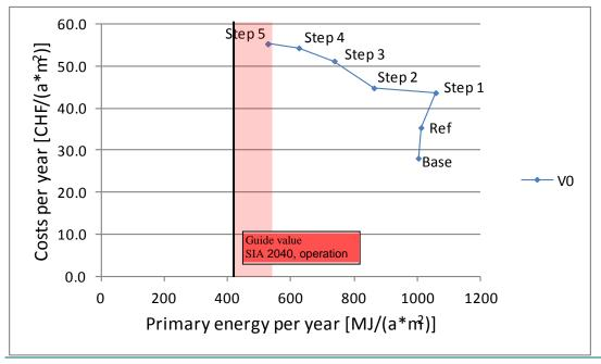
Figure 28: Yearly costs as a function PE efficiency increase due to the strategy steps of the "GHG oriented" strategy compared to guide value "operation" and "operation+construction" of SIA 2040.
