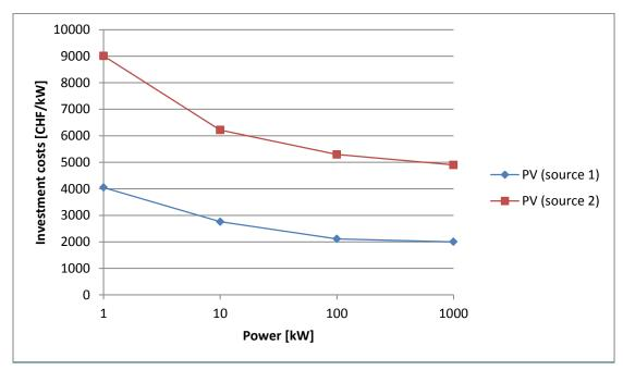
Figure 16: Two different scenarios of the investment costs of PV as a function of installed power
