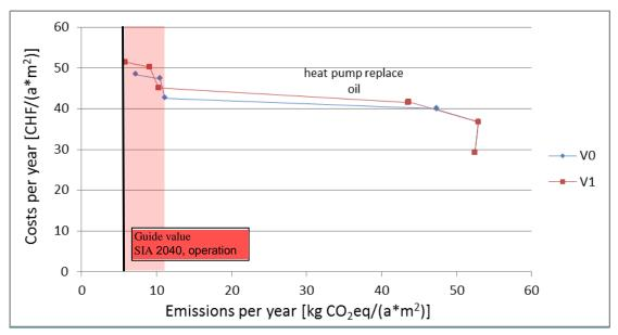
Figure 40: Yearly costs as a function of GHG emissions due to the strategy steps of the each strategy variant compared to guide value "operation" and "operation+construction" of SIA 2040.
