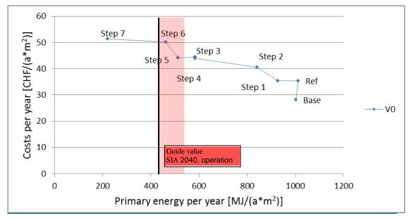
Figure 33: Yearly costs as a function PE efficiency increase due to the strategy steps of the "PE oriented" strategy compared to guide value "operation" and "operation+construction" of SIA 2040.
