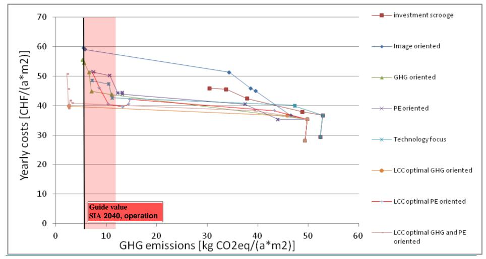
Figure 58: Yearly costs as a function of GHG emissions due to the strategy steps of the each main strategy (applied to the base case building from the construction period 1975-1990) compared to guide value "operation" and "operation+construction" of SIA 2040.
