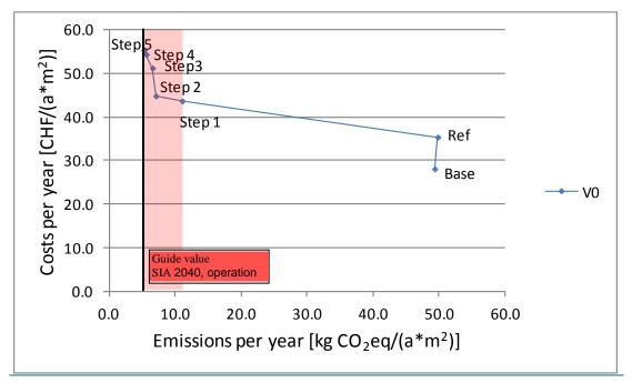
Figure 27: Yearly costs as a function of GHG emissions due to the strategy steps of the "GHG oriented" strategy compared to guide value "operation" and "operation+construction" of SIA 2040.
