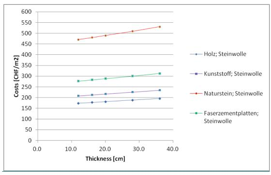
The cost level of ventilated façade is usually higher as compared to the compound façade. Likewise costs are increasing as a function of insulation thickness (see Figure 9).
