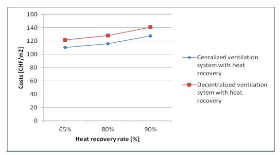
Figure 11: Investment costs of ventilation systems with heat recovery for a multifamily house as a function of heat recovery rate
