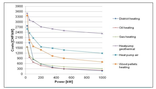
Figure 12: Investment costs<sup>11</sup> of different heating systems as a function of installed thermal power
