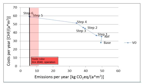
Figure 22: Yearly costs as a function of GHG emissions due to the strategy steps of the "image oriented" strategy compared to guide value "operation" and "operation+construction" of SIA 2040.
