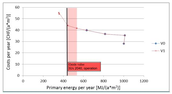
Figure 46: Life cycle costs as a function of PE use due to the strategy steps of the each strategy variant compared to guide value "operation" and "operation+construction" of SIA 2040.
