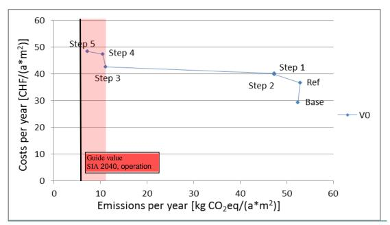
Figure 37: Yearly costs as a function of GHG emissions due to the strategy steps of the "technology focus" strategy compared to guide value "operation" and "operation+construction" of SIA 2040.
