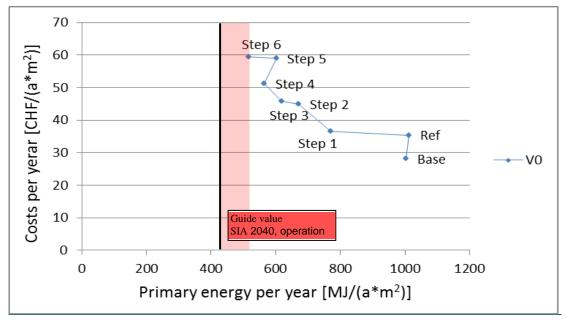
Figure 23: Yearly costs as a function PE efficiency increase due to the strategy steps of the "image oriented" strategy compared to guide value "operation" and "operation+construction" of SIA 2040.
