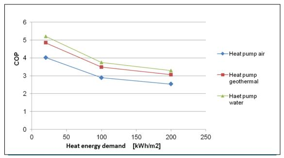
Figure 13: Seasonal energy-efficiency factor (annual COP) of heat pump heating systems as a function of the building efficiency
