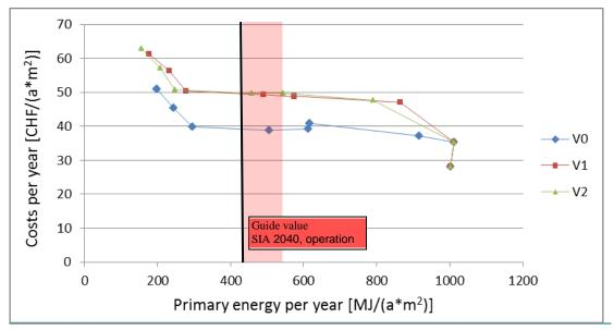
Figure 51: Yearly costs as a function of PE use due to the strategy steps of the each strategy variant compared to guide value "operation" and "operation+construction" of SIA 2040.
